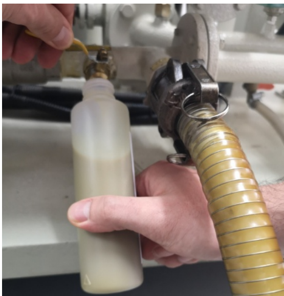
Figure 29. Sampling of the hydraulic oil with continuous flow, after drainage
