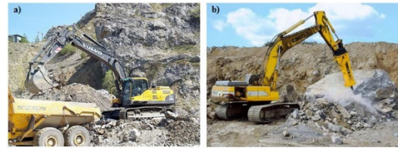
Figure 7. Single-bucket excavators in the mines of rock raw materials carrying out: a) loading, b) shredding oversized lumps ([21])
