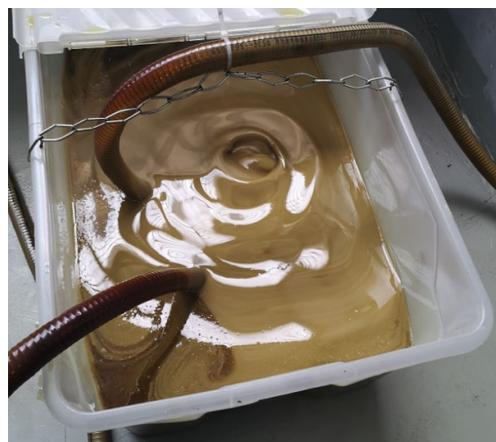
Figure 26. Test batch of hydraulic oil after the recirculation in the storage tank
